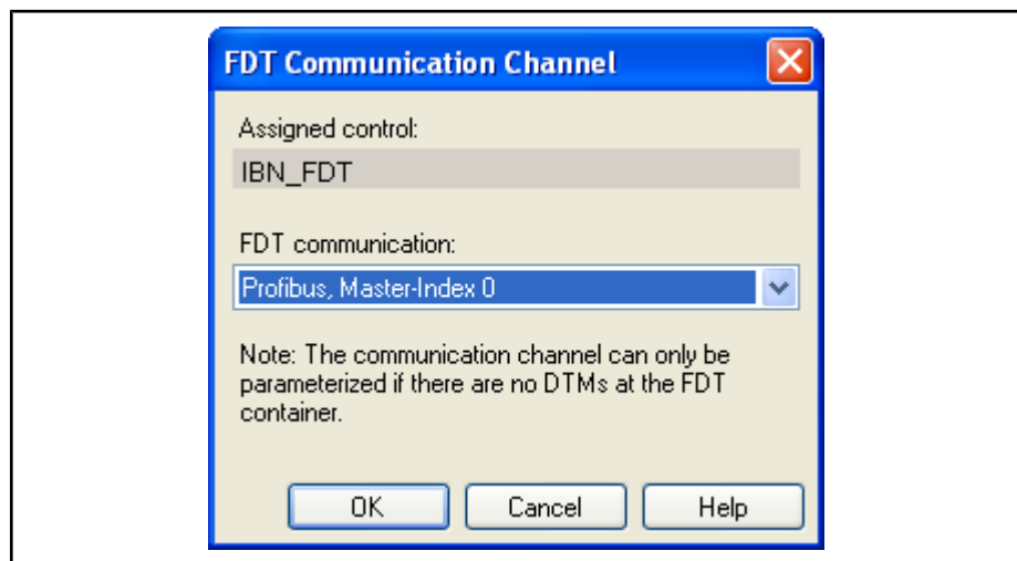
Fig.5-147: Setting the FDT communication channel
