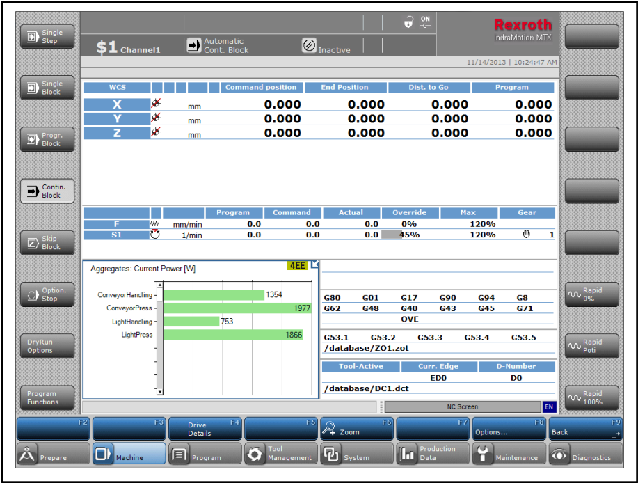
Fig. 8-7: Output power of the ancillary components
