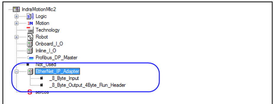
Fig. 7-27: EtherNet/IP adapter (engineering)
