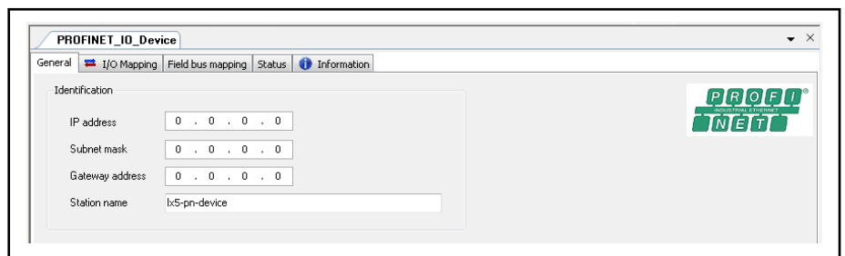
Fig. 6-51: Profinet I/O device - Tab "General"
