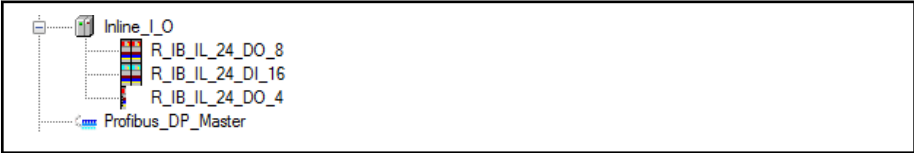
Fig. 12-6: Inline object with three modules (example)
