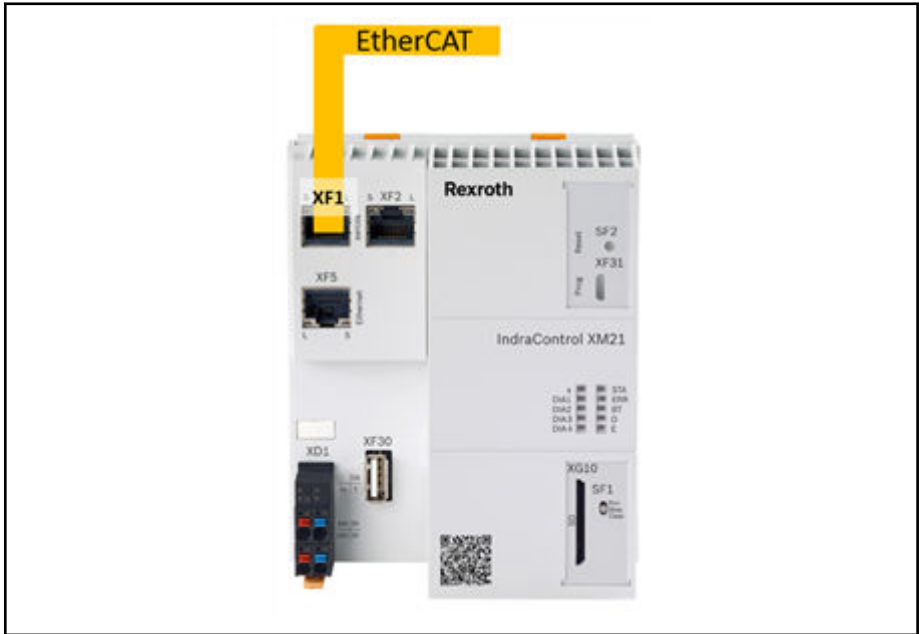
Fig. 8-20: EtherCAT cabling at the IndraControl XM21/XM22
