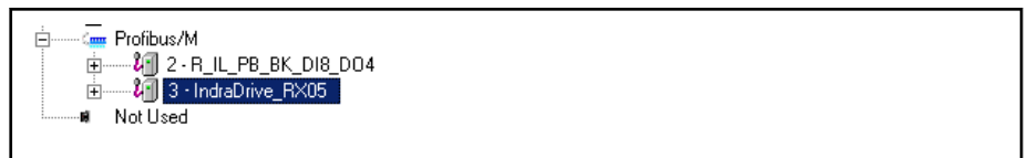
Fig. 4-26: Entering IndraDrive as Profibus device
