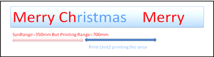
Fig. 4-86: Printing unit 2 for printing the blue area
