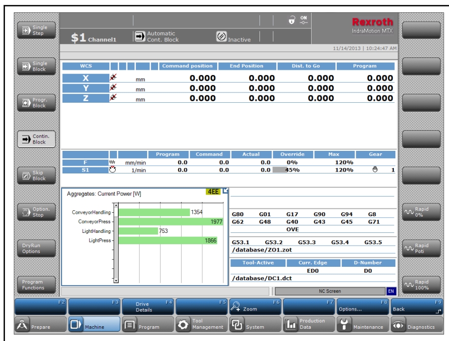
Fig. 10-12: Output power of the ancillary components
