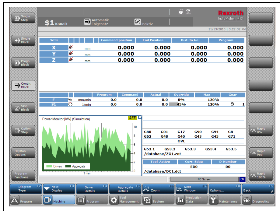
Fig. 10-10: Overall power (as timeline)
