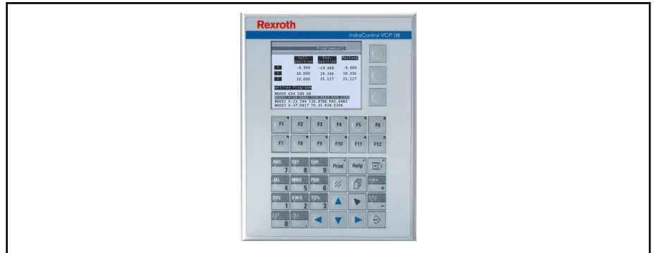
Fig. 9-3: VCP 08 small operator panel
