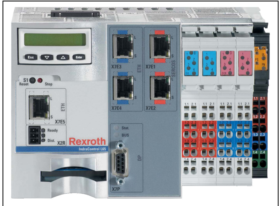
Fig. 5-1: IndraControl L65 control
