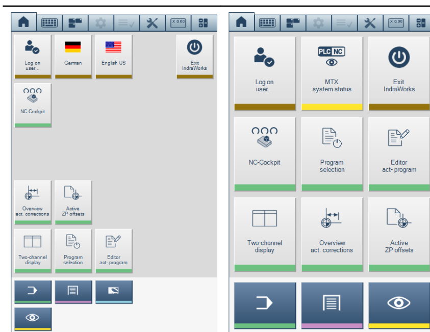
Home Control with small tiles and Home Control with large tiles and operating area keys
