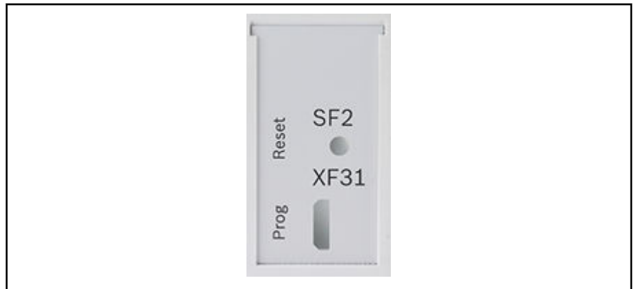
Fig. 4-2: Position of the reset button
