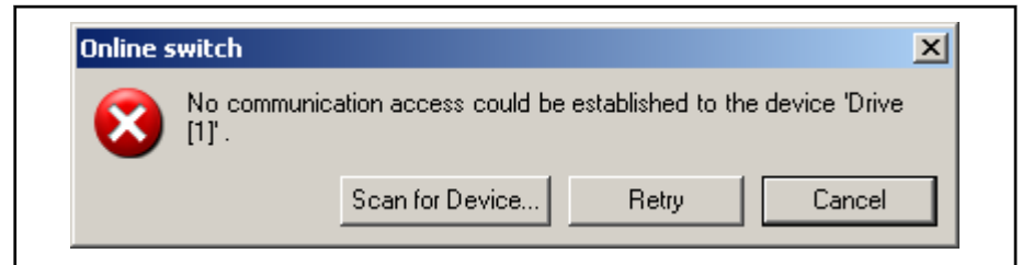
Fig. 3-41: Online switch (communication link not possible)
