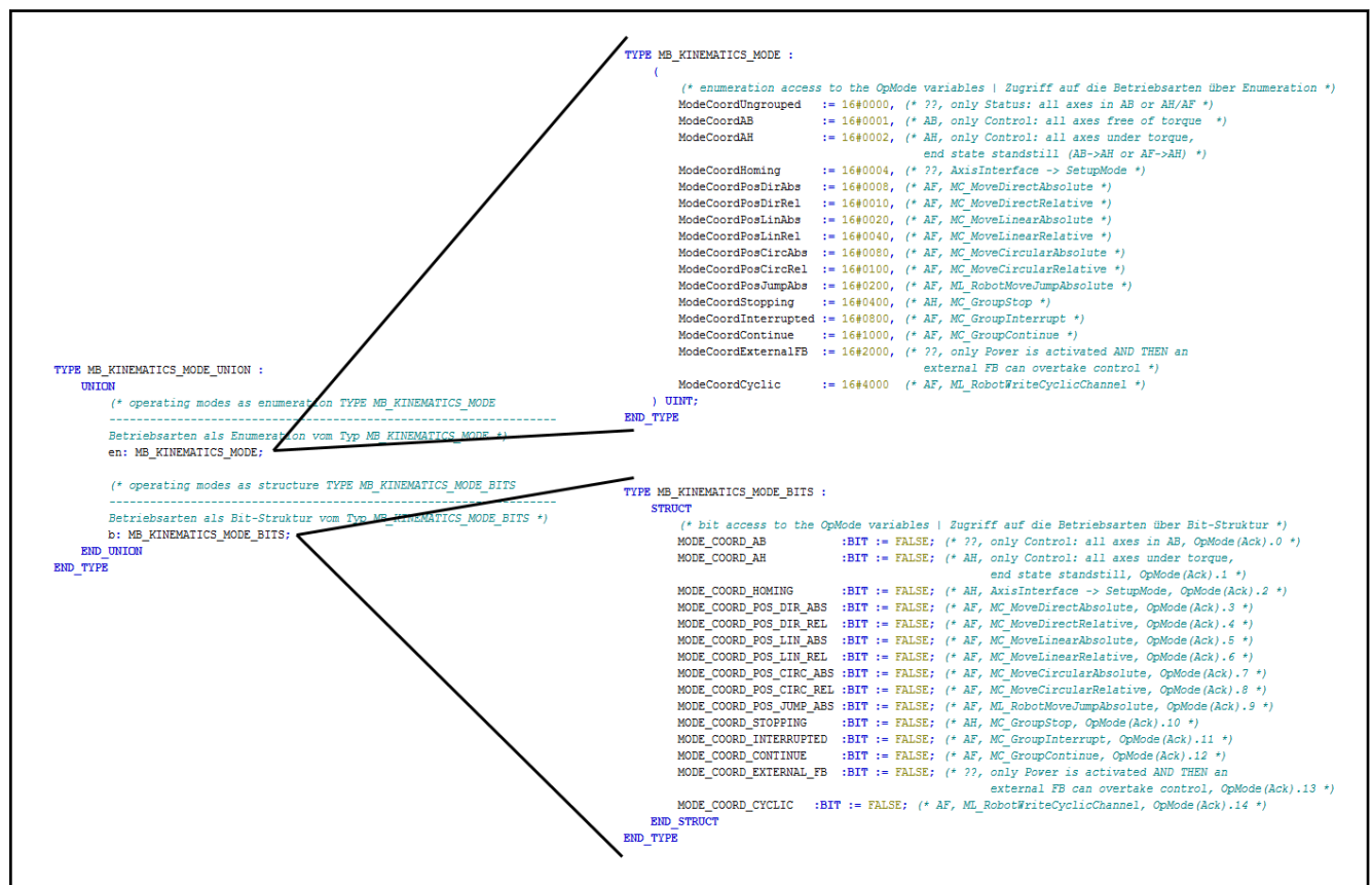
Fig. 17-74: Data type MB_KINEMATICS_MODE_UNION with MB_KINEMATICS_MODE and MB_KINEMATICS_MODE_BITS
