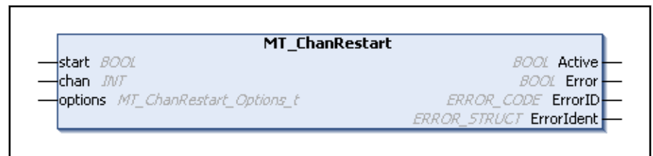
Fig. 12-5: MT_ChanRestart function block
